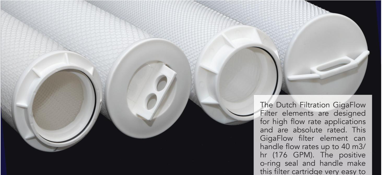
The Dutch Filtration GigaFlow Filter elements are designed for high flow rate applications and are absolute rated. This GigaFlow filter element can handle flow rates up to 40 m<sup>3</sup>/hr (176 GPM). The positive o-ring seal and handle make this filter cartridge very easy to install and remove from its filter housing. The full GigaFlow element are thermally welded and available in 1 – 150 micron. The GigaFlow is available in Glass Fiber as well as full Polypropylene.
