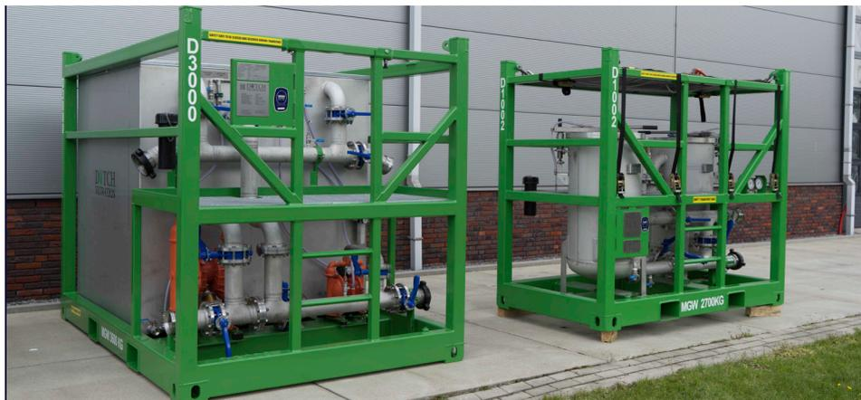
The Dutch Filtration dual mixing slurry skid is a complete unit for pre-coating and to body feed the filter press. The unit is complete with 2 mixing tanks, both 2.7 m<sup>3</sup>, air driven pre-coat and body feed pump. The frame is equipped with a working platform to safely and easily add filter aid (DE media) into the mix tanks.
