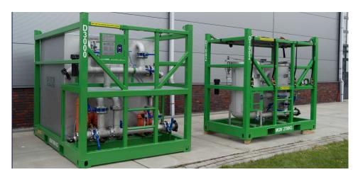
The Dutch Filtration dual mixing slurry skid is a complete unit for pre-coating and to body feed the filter press. The unit is complete with 2 mixing tanks, both 2.7 m<sup>3</sup>, air driven pre-coat and body feed pump. The frame is equipped with a working platform to safely and easily add filter aid (DE media) into the mix tanks.
